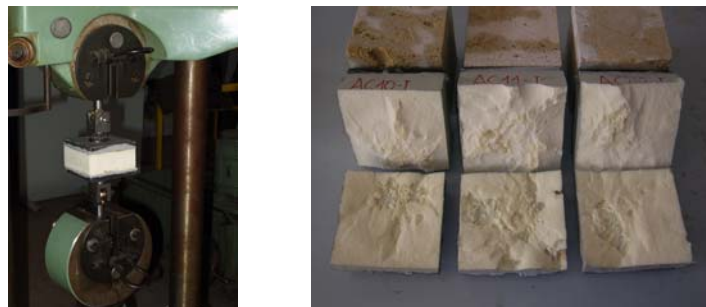
Fig. 2.9.11 - Tensile test and type of failure (PUR)
