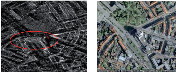
Figure 8. Example of layover of a high building on Hannover TSX image (left) and the same building in an aerial image (right)
