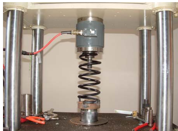
Fig. 5: Rear carriage spring during the test.
