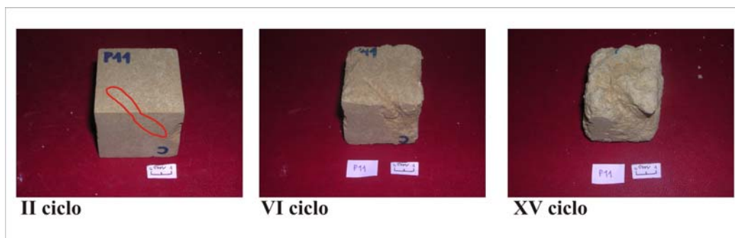
Fig. 3 - Loss of material around "skolithos" during II-VI-XV salt crystallization cycle.
