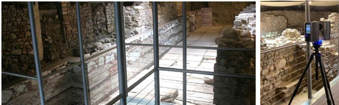
Fig. 8: (a) The archaeological area of Piazza Italia, Reggio C; (b) Scanning by Faro Focus 3D S 120.
