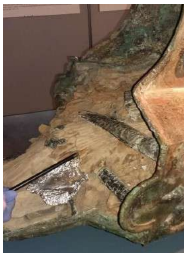
Fig. 4. Core sampling of the wooden part of the Acqualadroni rostrum
