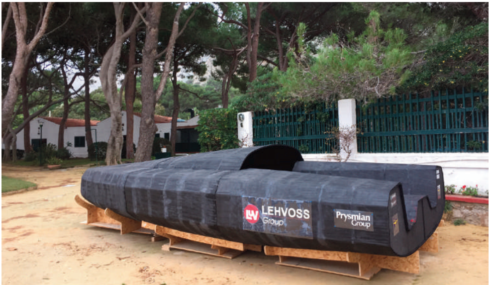
Fig. 16 - Mini 6.50 made entirely with additive manufacturing, Palermo 2018.
