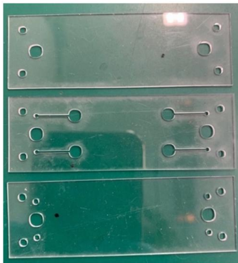
Figure 17 PMMA layers (0.5 mm thick) employed for the fabrication of the burst test device. The middle layer incorporates a microchannel leading to a circular chamber (4 mm diameter), while the external layers provide sealing and host the inlet/outlet ports for tubing connection.
