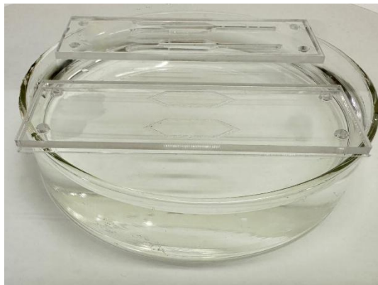
Figure 14 Solvent vapour polishing of engraved PMMA layers. The laser-machined substrates were suspended above a chloroform bath in a glass Petri dish to expose the engraved regions to solvent vapours, thereby restoring surface smoothness and optical clarity.
