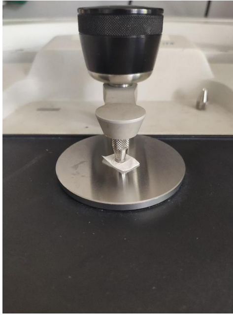
Figure 27 FTIR analysis of PLA scaffolds performed with a Thermo Scientific spectrometer. Samples were analyzed before and after integration into the microfluidic devices to monitor potential structural modifications.
