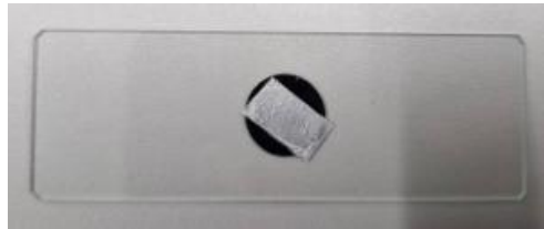
Figure 24 Membrane adhered to the glass slide with carbon tape
