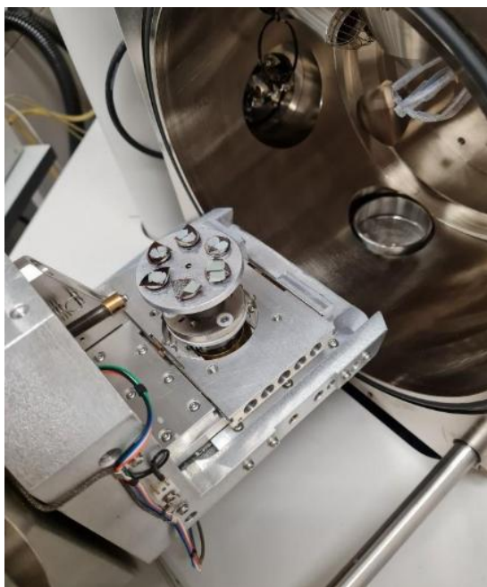
Figure 23 Scanning electron microscope (SEM) sample holder with electrospun PLA scaffold specimens mounted on aluminium stubs and coated for imaging. The system is shown inside the SEM chamber prior to analysis
