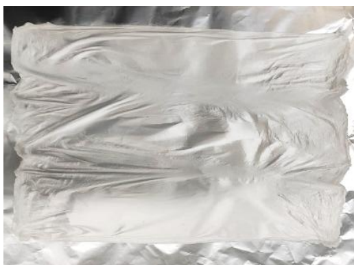
Figure 8 Representative image of an electrospun PLA fibrous mat ( \sim 20 \times 30 cm) after 180 min of electrospinning and 48 h drying under a fume hood.
