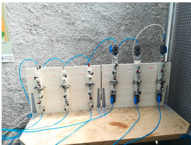
Fig. 2. Representation of the experimental setup, showing the six columns filled with zeolite.
