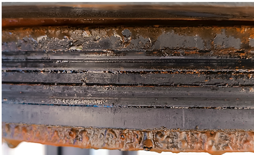
Fig. 9. Detail of the sealing system showing quad-rings.
