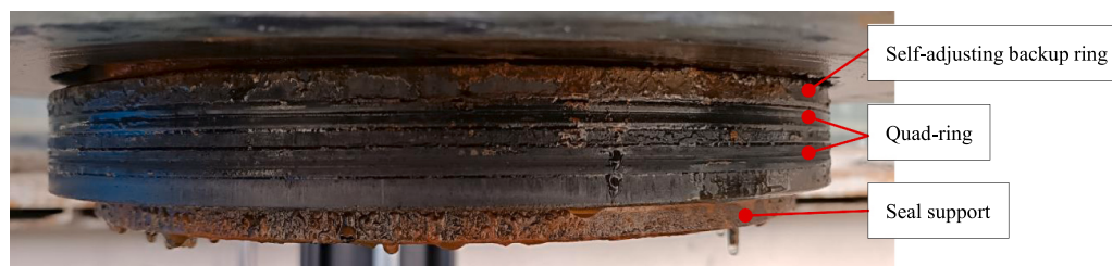
Fig. 8. Sealing system of the prototype after testing.
