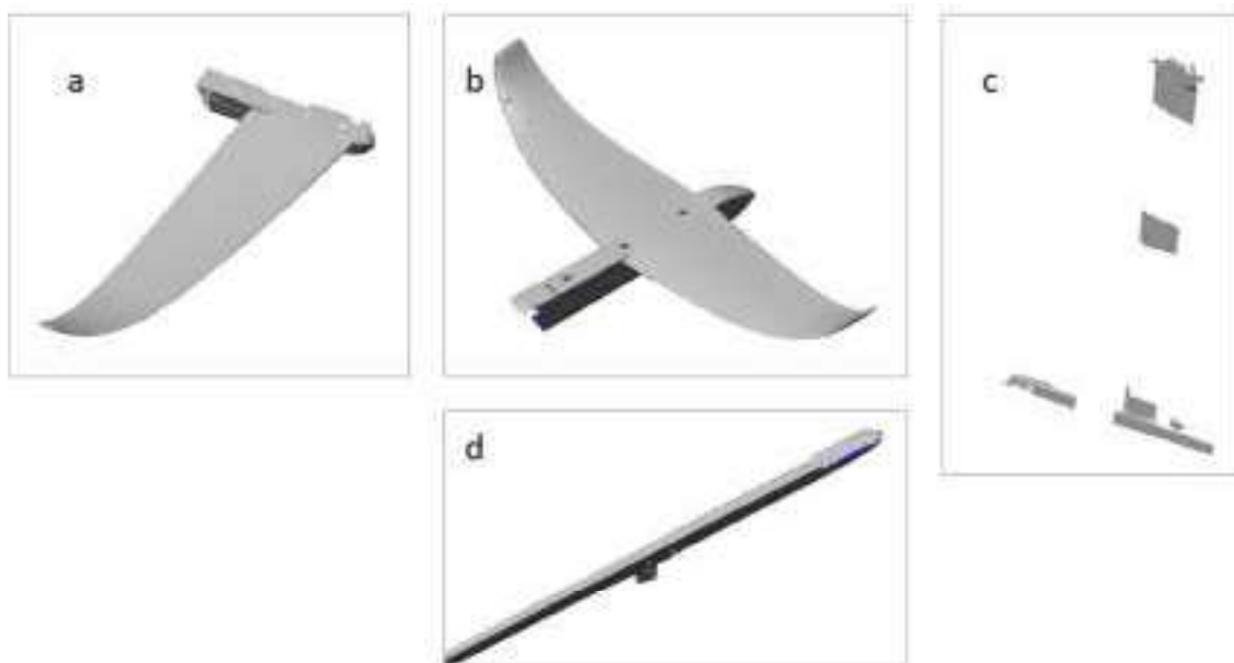
Fig. 2. Meshes generated from 3D scans of the iQFOiL components: a) Front; b) Back; c) Mast; d) Fuselage.
