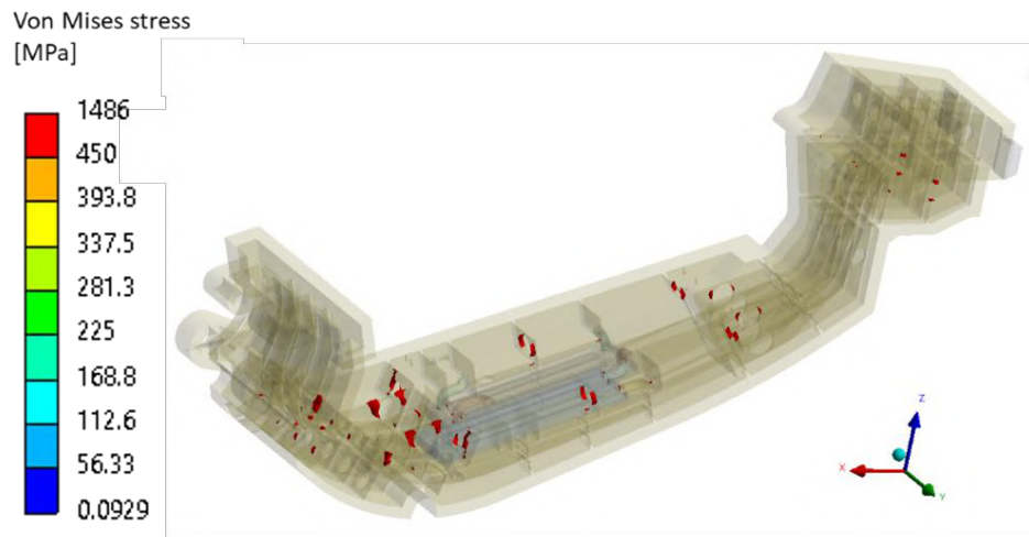
Figure 3.8 Most stressed regions of the model.
