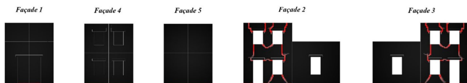
Fig. 7 Principal tensile strain distribution (max 0.01) obtained for 75% shaking table capacity, considering the Y-component
