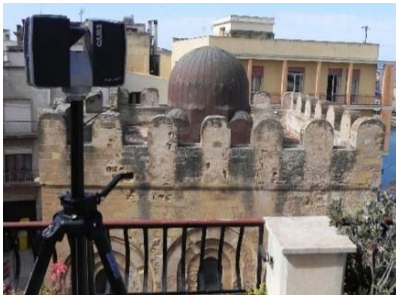
Figure 4: TLS acquisition of the external part of the roof.
