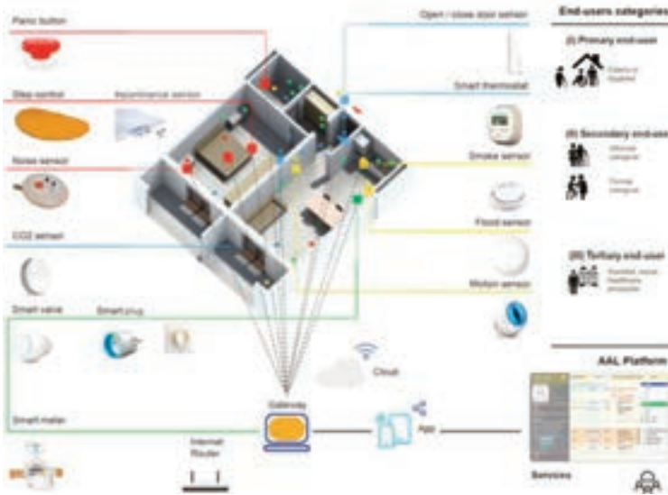
Fig. 27 | Model of the assisted house (AAL) for fragile users, IoT technologies and interaction with the ICT service platform (credit: A. Mangiatordi, 2020).
