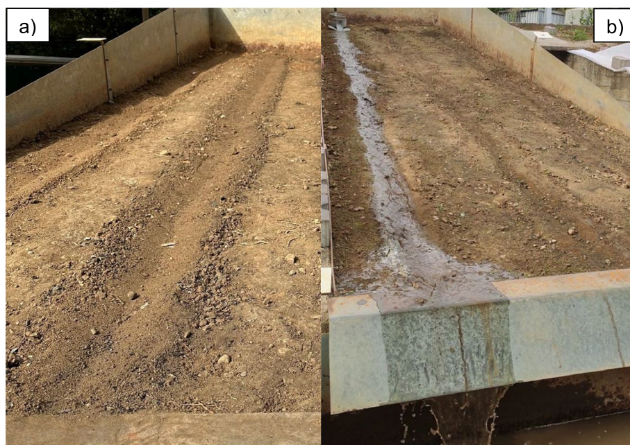
FIGURE 2 | View of the preferential path (a) and flow moving in the rill (b).
