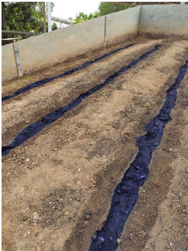
FIGURE 3 | Water tracks inside the channels marked by using a Methylene blue solution as a dye tracer.
