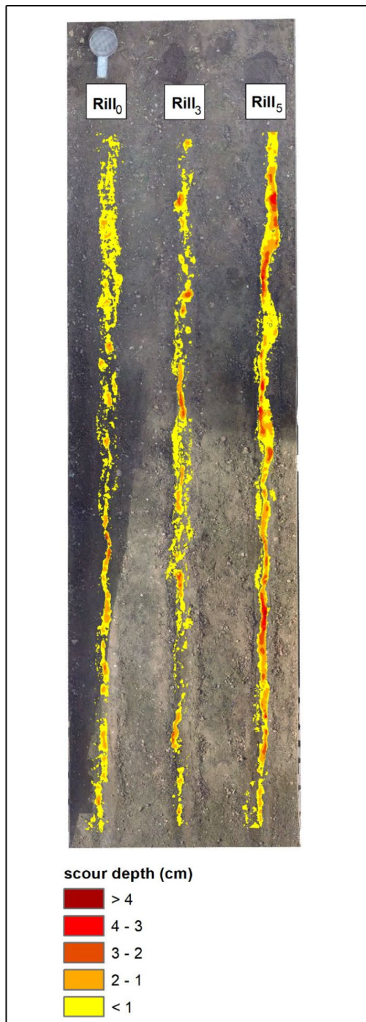
FIGURE 5 | DEM of difference (DoD) obtained for the rills with a biochar concentration of 0% (rill 0 ), 3% (rill 3 ) and 5% (rill 5 ).
