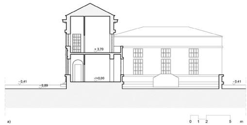
Fig. 05. Enrico Del Debbio, Casa del Balilla in Enna: a) section A-A; b) digital three-dimensional model, perspective section A-A (graphic elaborations by the author).
