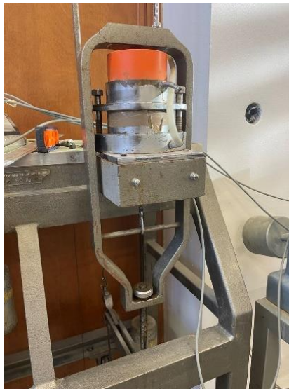
Fig. 13) Consolidometer; the 1D compression apparatus.
