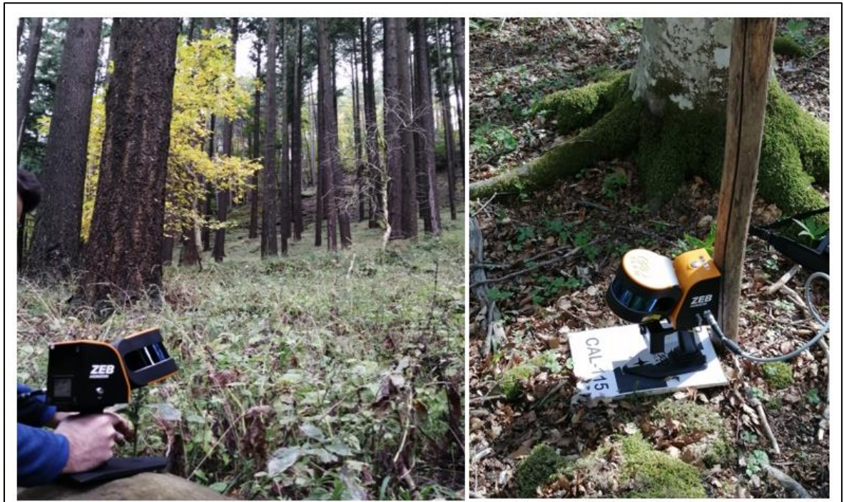
Figure n. 15 - GEOSLAM ZEB HORIZON™ Hand Held Mobile Laser Scanner (HLS)
