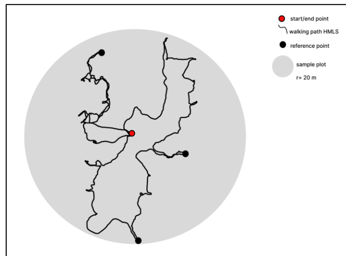
Figure n. 20 - Scheme of walking path during HLS applied into the fifth case study.
