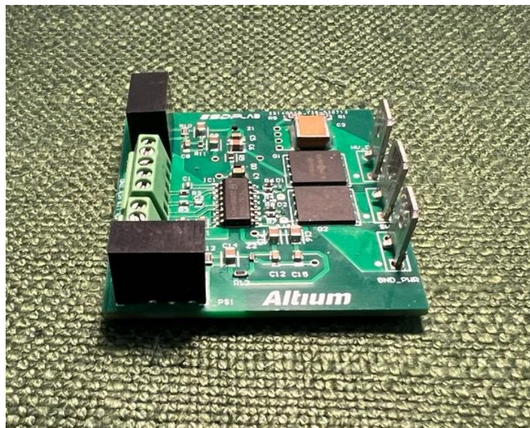
FIGURE 2.15: GaNPower-based Half Bridge Prototype
