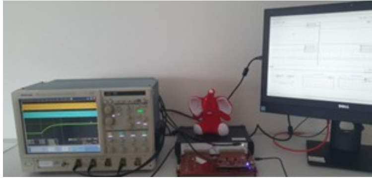
FIGURE 3.26: Experimental testbench with Typhoon HIL 404 and TI C2000 MCU for DAB control validation.
