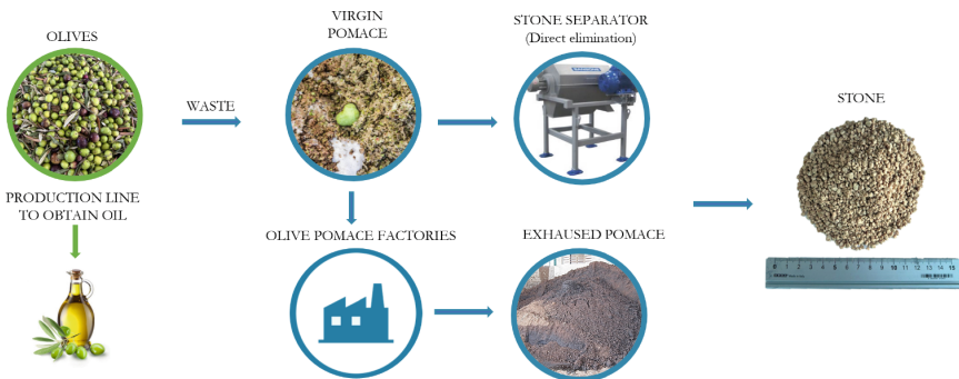
Fig. 2. Diagram of the stages from which olive kernel is derived—© 2024, the authors.
