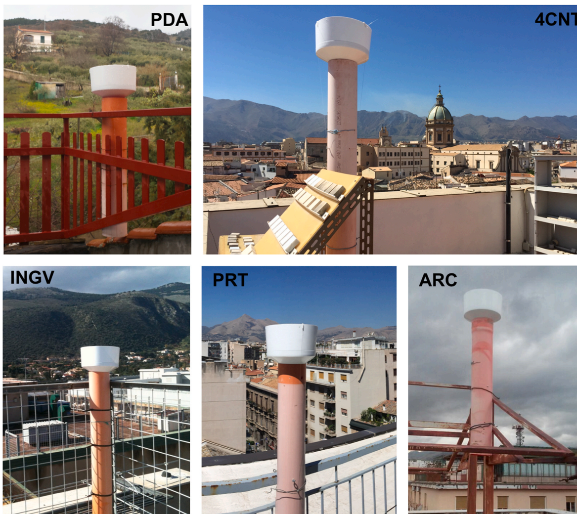
Fig. 2. Photos of the rain gauges installed in the different sampling sites.
