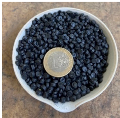
Fig. 3. The graphene-based additive used in this study.
