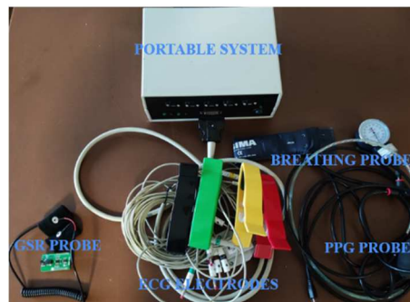
Fig. 3. Overview of the portable biomedical system, alongside with ECG and GSR electrodes, PPG and breathing probes.
