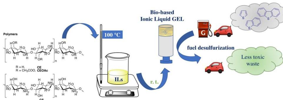
**Figure 1:** Biopolymer structures, schematic representation of IL gel preparation and of fuel desulfurization.
