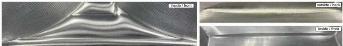
Fig. 27 Pronounced pillow effect with visible toolpath marks (left) and fracture at the discrete angle change (right). Results from ULisboa EXP #1
