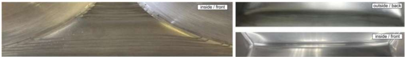
Fig. 28 Reduced pillow effect (left) without fracture at the discrete angle change (right). Results from ULisboa EXP #4
