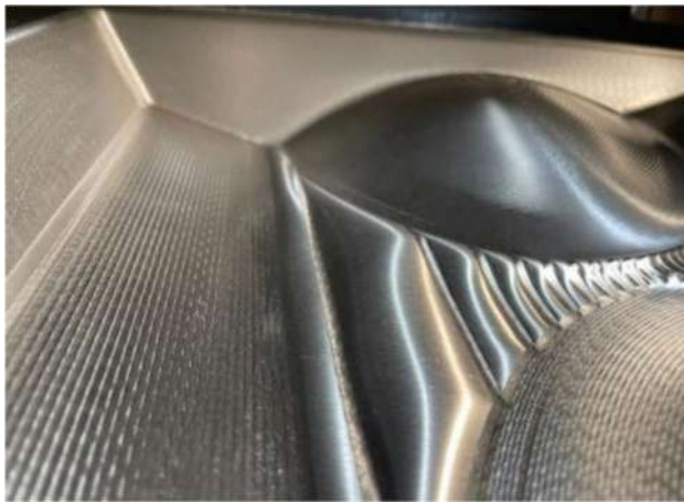
Fig. 17 The pronounced pillow effect observed in the flat waist area (zone D)
