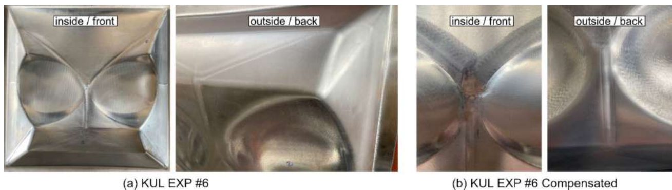
Fig. 52 Edges formed in previous steps are, even after forming the area again, still visible in the final shape
