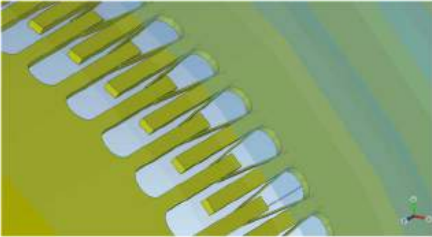
Fig. 2.25. View from inside of the RF shielding with small fingers between the teeth.
