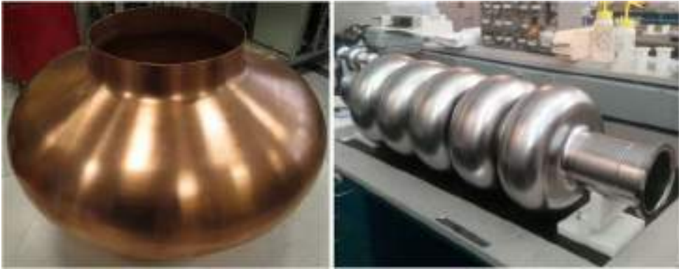
Fig. 3.16. Left: A FCC seamless single-cell 400 MHz Cu prototype cavity for Nb on Cu thin-film coating, fabricated at INFN Legnaro National Laboratory (Italy). Similar cavities will be used for operation at the Z pole. Right: A prototype FCC five-cell 802 MHz bulk-Nb cavity for t\bar{t} operation, fabricated and tested at Jefferson Lab (USA) [304].
