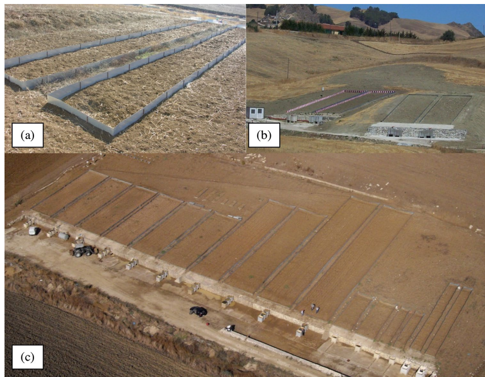
Fig. 1 View of the a unit plots, b 22% and 26% sloping plots, and c 14.9% sloping plots of the Sparacia experimental area
