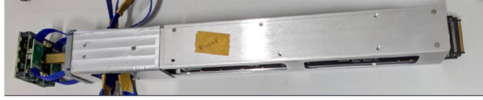
Figure 4: Single module picture composed by 64 SiPMs.
