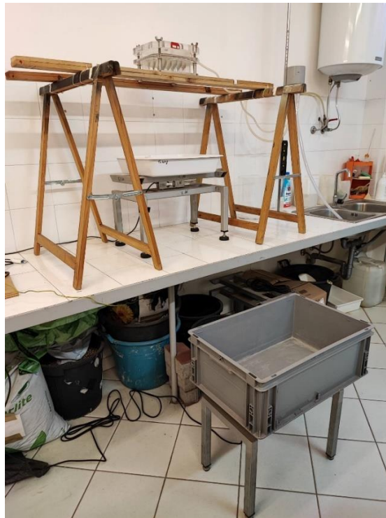
Figure 14. Experimental installation: at the top the needle simulator, on the counter, and at the bottom the two load cells for measuring the water content and volumes drained from the microcosm of the green roof.
