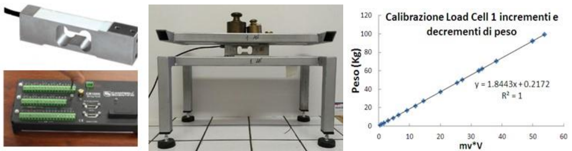
Figure 15. Load cell and acquisition system. On the right the experimental calibration report for cell no. 1.
