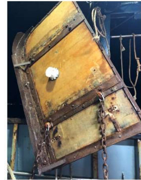
Figure 2: Reference scheme for Inertial Measurement Unit (IMU) displacement on the surface of the otter board and interpretation of inclination angles ( \Phi , \Psi and \Theta ) across the three main axis of the gravity vector g . On the right side the pictures of the watertight lid used to secure the sensor to the door's surface and the final configuration once attached. IMU unit contained a three-axial accelerometer and gyroscope used to measure the main acceleration forces and changes in angular velocity and estimate the inclination of the otter board during towing activity.
