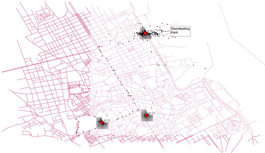
Fig. 1 Example of a GPS track (black points) and stops derived from the DBSCAN algorithm (red stars) for a cruiser in the municipality of Palermo. The top numbers in the circular indicate which stop has been first visited. The circular's bottom numbers indicate the times spent in minutes at each stop (colour figure online)
