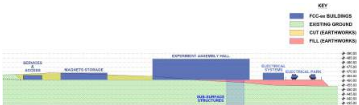
Fig. 1.26 Preliminary simplified cross-section of PD surface site
