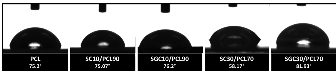
Figure 4.30: Contact angle measurements on SC/PCL, SGC/PCL, and neat PCL film obtained by hot pressing.
