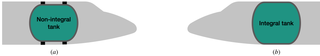
Figure 3.1: a) Non-integral tank architecture in which the pressure vessel is structurally independent from the aircraft fuselage. The tank experiences a pressure differential defined by the difference between the internal tank pressure and the internal fuselage pressure vs b) integral tank in which the walls are partially made by the aircraft fuselage structure. In this configuration, the tank is subjected to a pressure differential equal to the difference between the internal tank pressure and the external ambient pressure.
