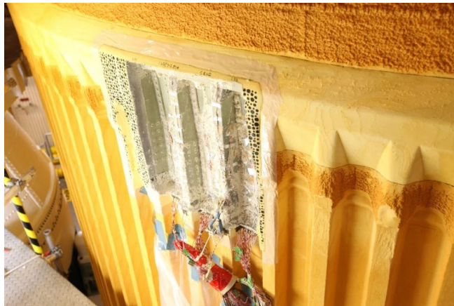
Figure 1.6: Detail of the Space Shuttle external cryogenic tank. Orange coated SOFI foam was used to insulate LH 2 and oxygen [3].
