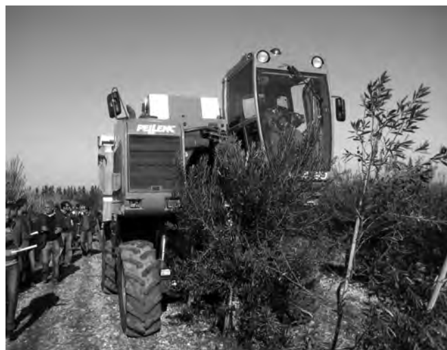
Fig. 2 - Vendemmiatrice. Fig. 2 - Grape-harvester.
