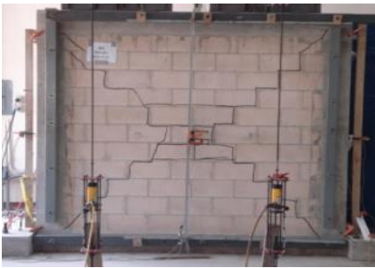
Concrete block masonry ( l/h = 1.0 )
