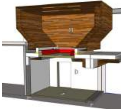
Figure 2. Details of mobile source room installation above the test floor (details without showing absorbing wool filling) and CLT slab installed between rooms.
