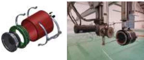
Figure 1. Underwater sound source: (Left) Schematic design assembly drawing, and (Right) picture of the mounting conditions used to measure its on-axis pressure response (before immersion in the water tank).
