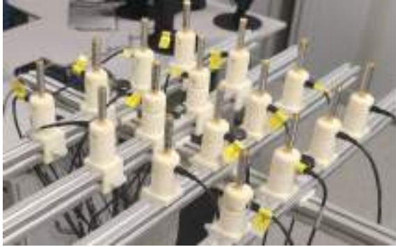
Figure 4. Rectangular array with Brüel&Kjaer type 4958 microphones.
