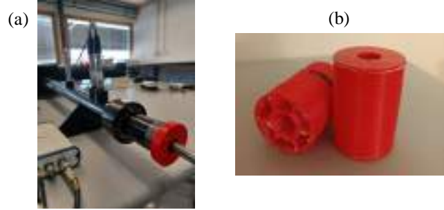
Figure 3. (a) Image of the implemented measurement setup. (b) Photograph of a printed AMM cell.
