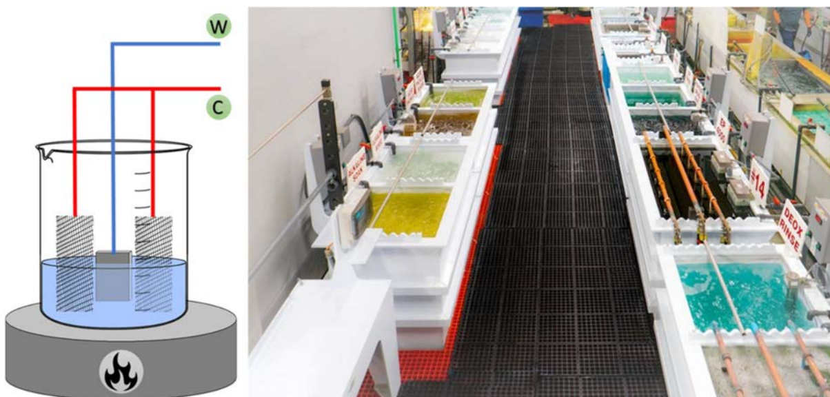
Figure 11. Scalable electrochemical surface treatments: laboratory-scale experimental setup (left) and industrial bath processing line (right).
