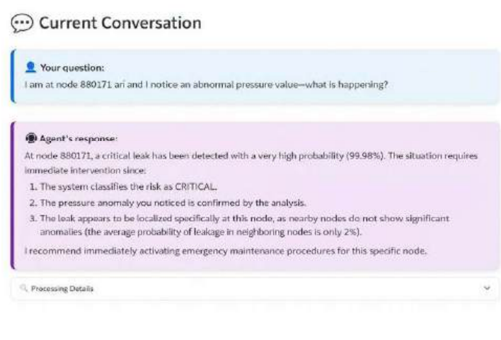
Fig. 20: System response with notification of a critical leak diagnosis in node 880171.
