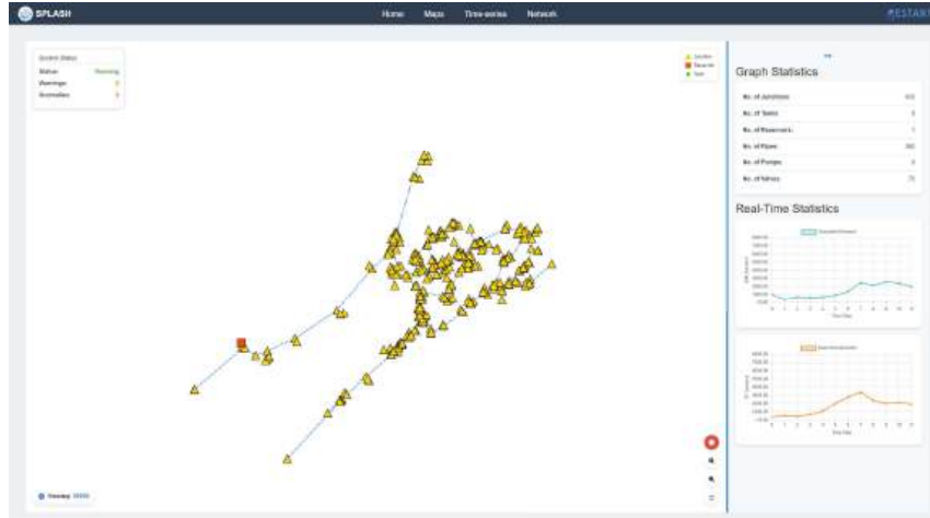
Fig. 18: SPLASH hydraulic simulation view, enabling comparison between real and modelled network states.
