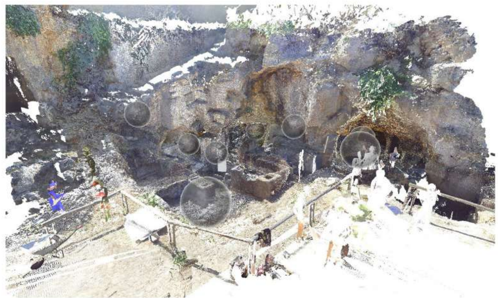
Figure 10. Faro Focus 3D S120 point cloud of the Latomia dei Niccolini; the gray spheres show the eight scanning positions.
