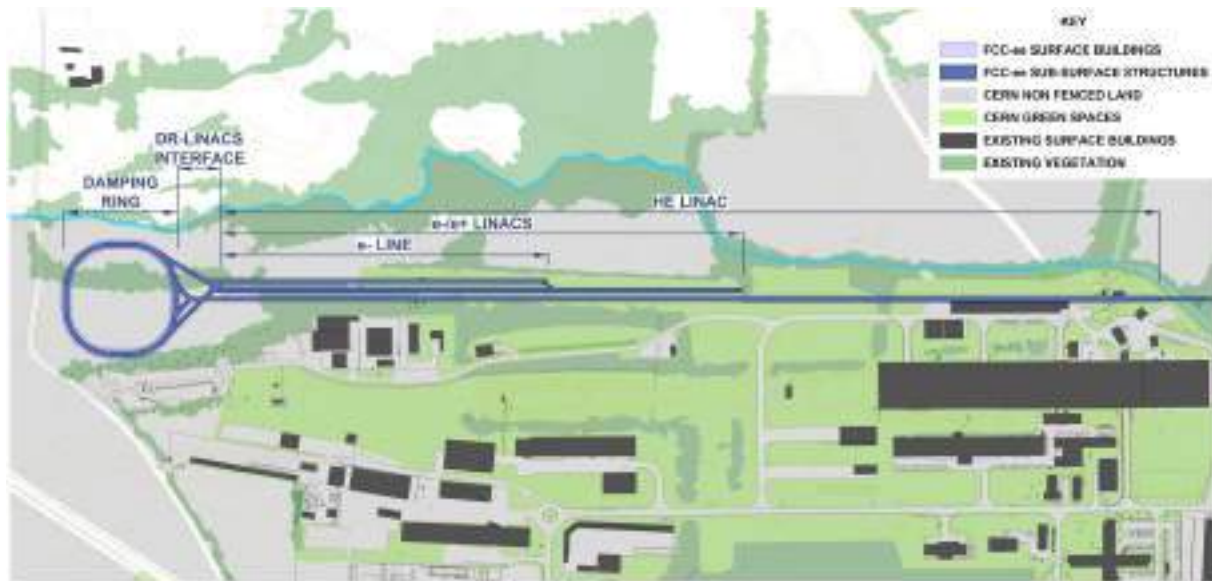
Fig. 7.35 Plan view of high-energy linac civil engineering
