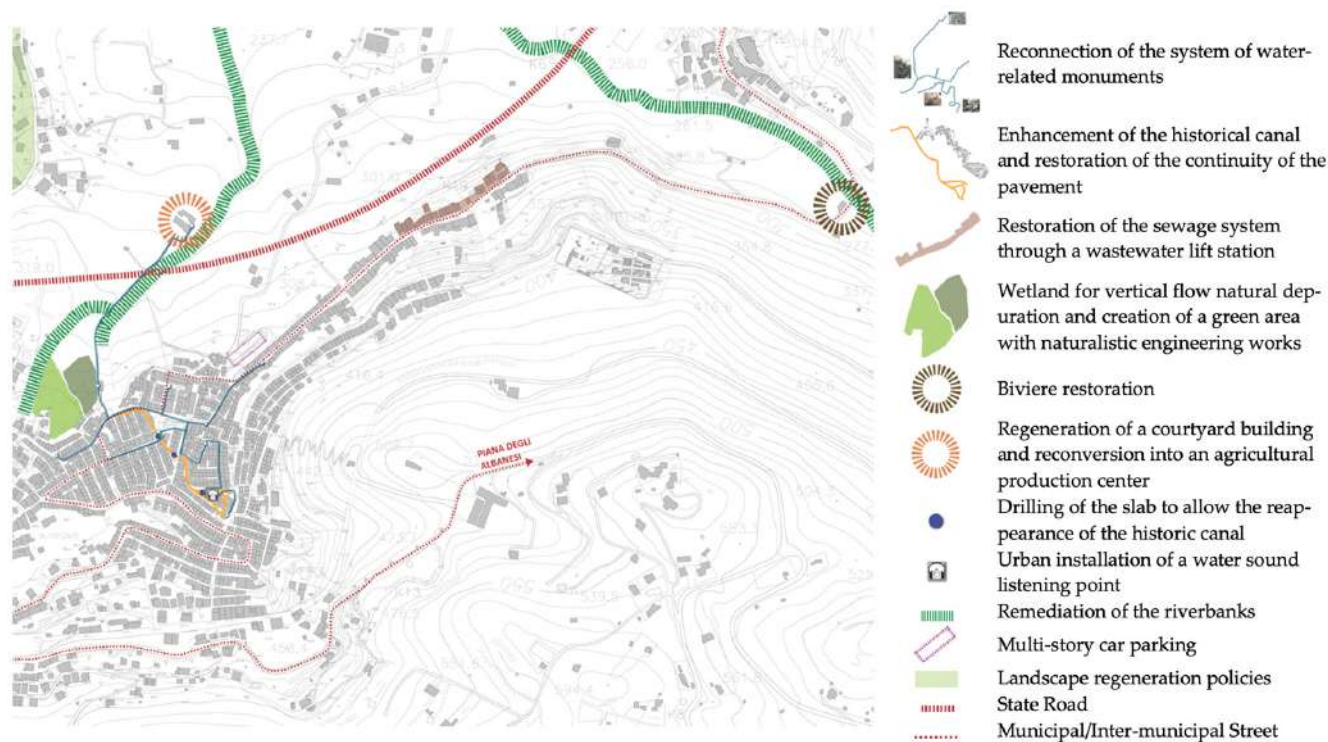
Figure 5. Circular water project for Altofonte. The project includes the restoration of architectural elements and urban redevelopment, riverbed reclamation actions, greening solutions, interventions to the sewerage network and recovery of historic canalizations (image elaborated by Arch. Nicolò Di Matteo).
