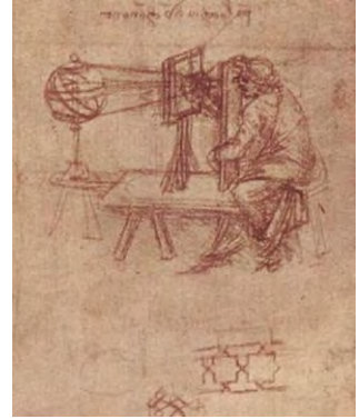
Fig. 5/ Illustrazione di una camera oscura. Da James Ayscough, A short account of the eye and nature of vision. Chiefly designed to illustrate the use and advantage of spectacles . London, 1755.
