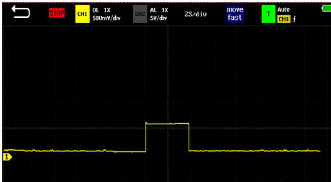
Figure 3. A screenshot from the oscilloscope connected to the test device of figure 2. It represents the effect of a dark soliton irradiated on the device, which determines the immediate increase of the electrical resistance of the overlapped layers, causing the voltage at the insertion point of the RC load resistance to rise by about 600 mV. The subsequent irradiation, after 4 s, with a bright soliton causes the quick collapse of the electrical resistance and the return of the device to its initial state.
