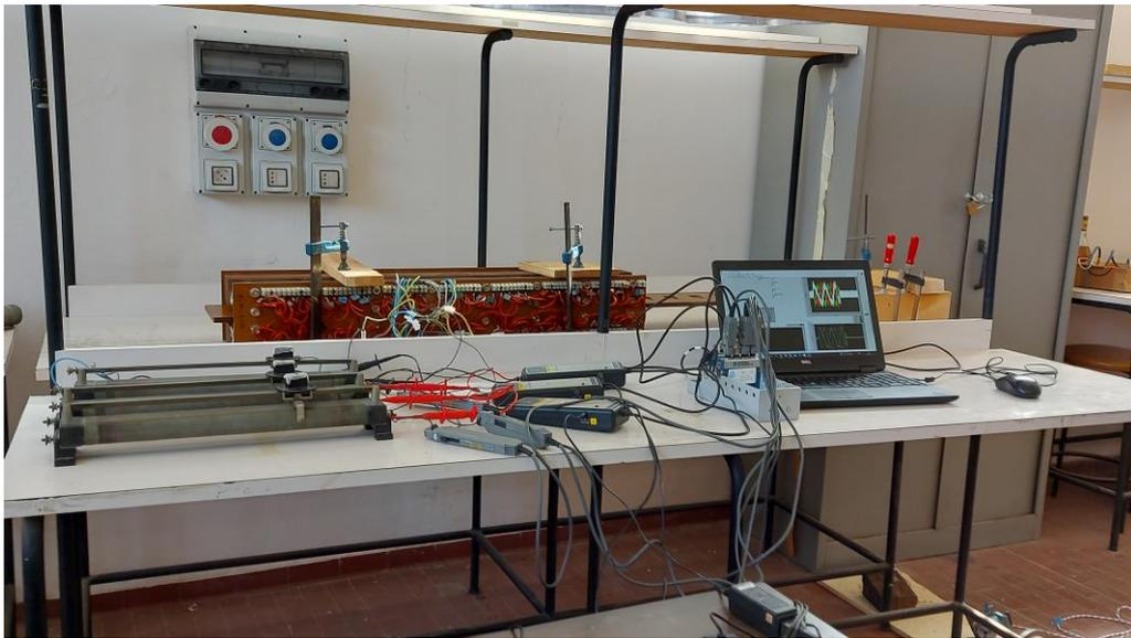
**Figure 92. Linear generator experimental tests**
