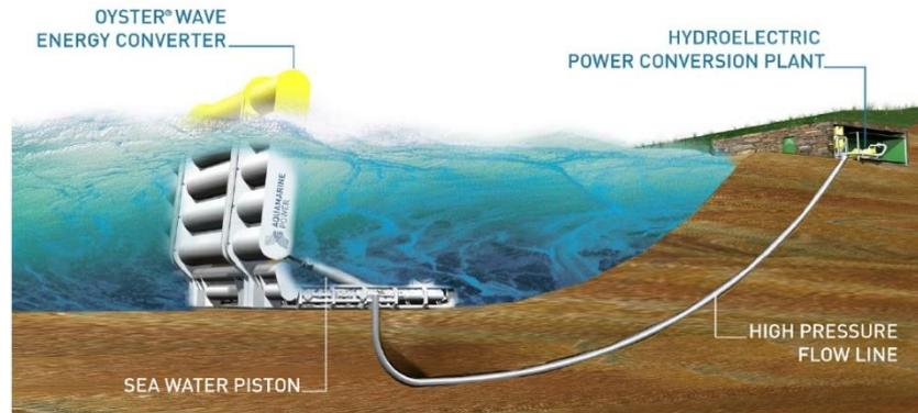
**Figure 27. Working principle of Oyster**
