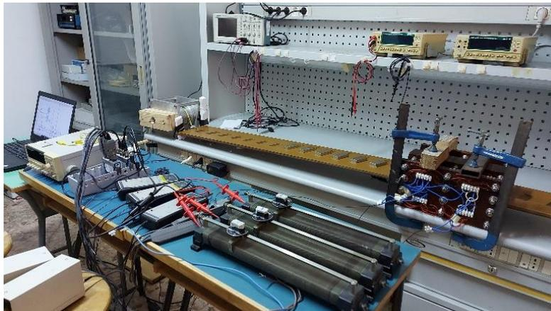
**Figure 109. Ironless linear generator experimental tests**
