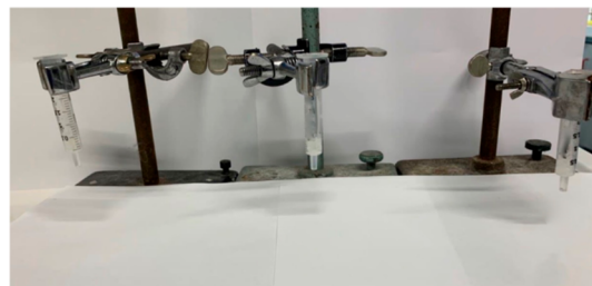
Figure 9. Picture of gel-loaded syringes for sequential adsorption of BPA from flowing aqueous phases.
