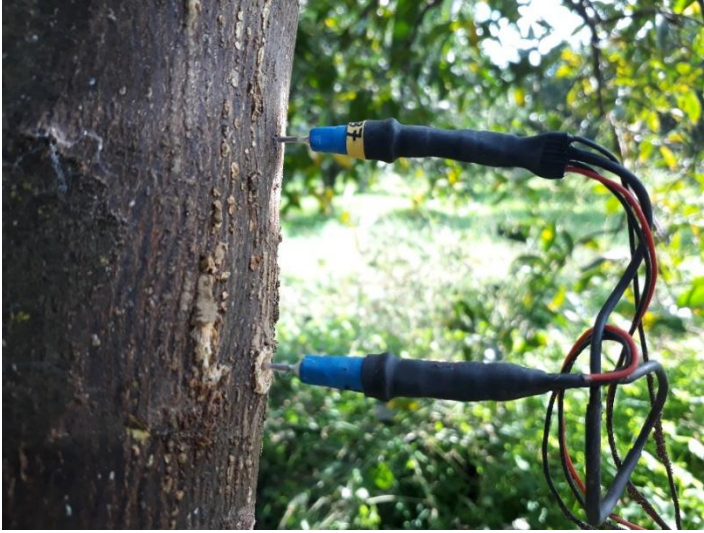
Fig. 5 Sap Flow sensors
