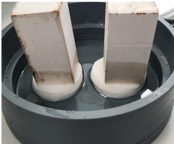
Fig. 4. Example of water absorption test
