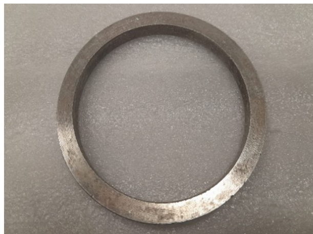
Figure 1. FeSi toroidal sample made by additive manufacturing using the L-PBF technique.
