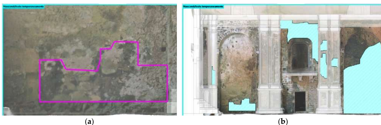
Figure 23. An example of contour tracing: (a) detail of fragmentation on surface layer; (b) the parametric families created accordingly.
